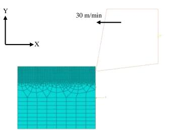
Figure 2: Finite Element model of the workpiece and the cutting tool.
