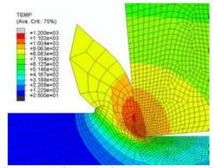
Figure 1: Material of the workpiece flows around the tool edge; no chip separation criterion is used [5].
