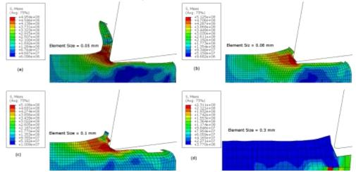
Figure 4: Effects of mesh size on the chip formation and its continuity.
